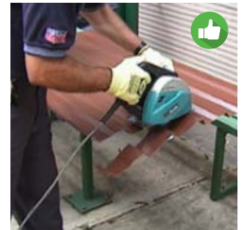
Use a cold metal cutting blade together with appropriate holding tools to ensure stable cutting and minimise burr formation
