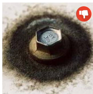
Inadequate or incompatible accessories can lead to ring around corrosion to the surface
