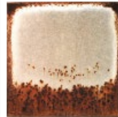
Galvanised steel Z275 (Heavy sign of Rust)
