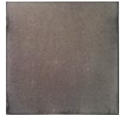
ZINCALUME® steel (No Sign of Rust)
